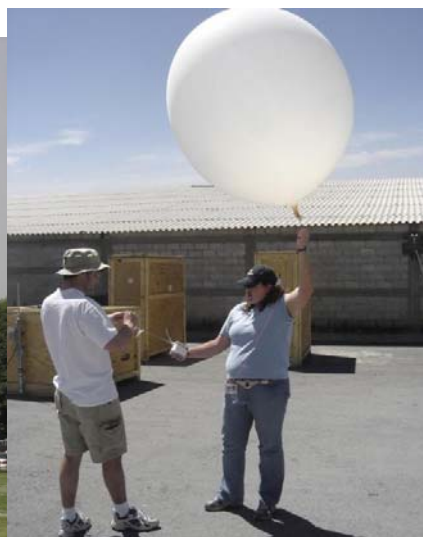
Left: Tethered balloon will be launched three times daily at the site (vertical profile of meteorological parameters and ozone)
