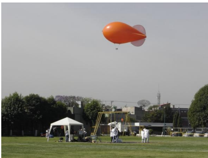
Left: Tethered balloon will be launched three times daily at the site (vertical profile of meteorological parameters and ozone)
